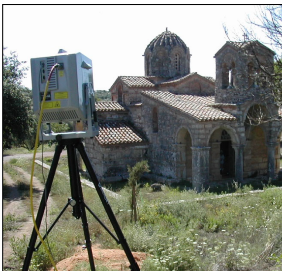
Static Terrestrial Laser Scanning
