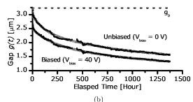
Figure 5. The measured (black) and fitted (red) results of the analog RF-MEMS varactor. (a) The measured capacitance.  $C_o$  is the initial capacitance. (b) The FEA-extracted gap.  $g_o$  represents the initial gap.
