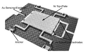
Figure 1. The confocal-microscopy image of the fabricated analog RF-MEMS varactor. The gap between the Ni plate and Au electrodes is  $3 \mu m$ . There are no dielectric layers in this varactor.
