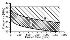
Figure 8. The simulated tuning range of the tunable RF-MEMS resonator. (I) The actual tuning range. (II) Based on conventional spring constant.
