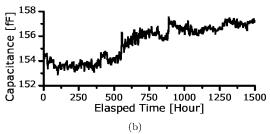
Figure 4. (a) The measurement uncertainty. (b) The measured long-term drift is less than 4 fF over 1,500 hours.
