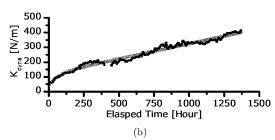
Figure 6. The measured (black) and fitted (red) spring constant. (a) Conventional spring constant. (b) Dynamic spring constant.
