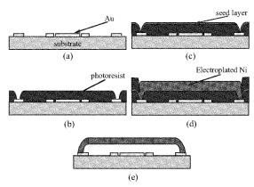
Figure 2. Fabrication process of the Ni analog RF-MEMS varactor.
