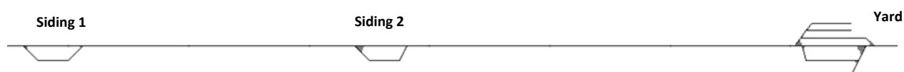
Figure 5.4. A simple scheme of sidings and yard located along the case study
