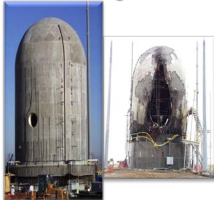
1/4-Scale Prestressed Concrete Containment Vessel Failure Test
