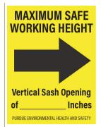
Left: This sticker shows the maximum height the sash can be safely opened - the sash should always be kept as low as possible and closed when not in use.
