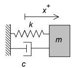
**Given:** The addition of damping to an undamped system causes the period to increase by 25 percent.
