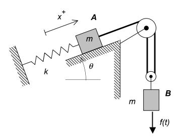
**Given:** Blocks A and B (having masses of m and 3m, respectively) are connected by a cable-pulley system as shown below. A spring of stiffness 3k is attached between A and ground. A second spring of stiffness k is attached between block B and ground. Let x describe the position of A, where the springs are unstretched when x = 0.
