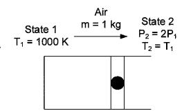
Calculate the entropy generation for air in the cylinder, in kJ/K. Assume a boundary temperature of 1000 K.
