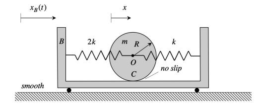
Use the following parameters in your analysis: m=200 kg,  $k=10{,}000$  N/m, b=0.1 m, and  $\Omega=15$  rad/s.
