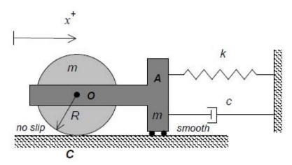
Use the following parameters in your analysis: m=4 kg, k=2250 N/m, R=0.1 m, c=60 kg/s, and  $v_0=8$  m/s.
