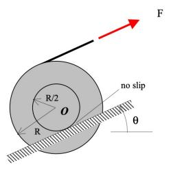
Use the following parameters in your analysis: m=40 kg, R=0.2 m, d=2 m, F=100 N,  $k_O=0.15$  m, and  $\theta=30^{\circ}$ .
