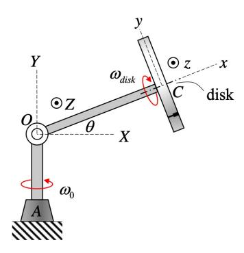
Use the following parameters in your analysis:  $\theta = 36.87^{\circ}$ ,  $\omega_0 = 4 \text{ rad/s} = \text{constant}$  and  $\omega_{disk} = 6 \text{ rad/s} = \text{constant}$ .
