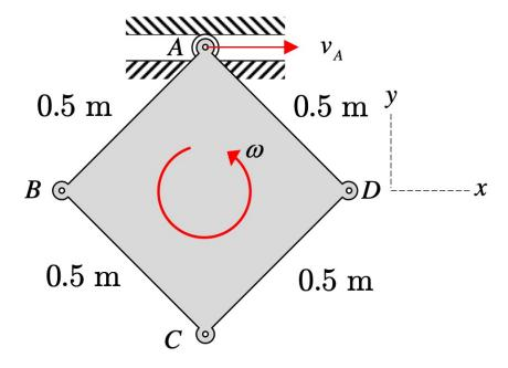
Use the following parameters in your analysis:  $v_A = 6$  m/s and  $\omega = 5$  rad/s (CCW).
