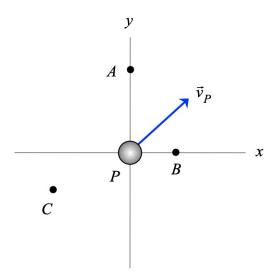
Use the following parameters in your analysis: m=5 kg,  $\vec{v}_P=\left(20\hat{i}+15\hat{j}\right)$  m/s and the following (x,y) coordinates for points A, B, C and P: A:(0,1.2) m, B:(0.9,0) m, C:(-0.4,-0.3) m, and P:(0,0) m.
