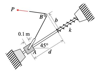
Use the following parameters in your analysis: m=28 kg, P=50 N, b=1 m, d=1.2 m and  $\Delta_{max}=0.02$  m.
