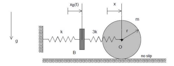
Use the following parameters in your analysis: m = 80 kg, k = 640 N/m, r = 0.25 m, b = 0.16 m, and  $\Omega = 10$  rad/s.
