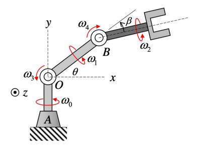
Use the following parameters in your analysis:  $\omega_0 = \omega_2 = \omega_4 = 0$  rad/s,  $\omega_1 = 2$  rad/s,  $\theta = 60^{\circ}$  and  $\dot{\theta} = \omega_3 = 1.5$  rad/s.
