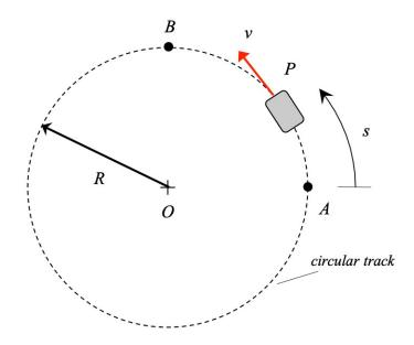
Use the following parameters in your analysis: b = 0.001/m, R = 500 m and  $v_A = 80 \text{ m/s}$ .
