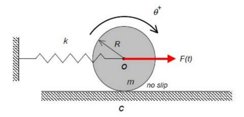
Use the following parameters in your analysis: m=2 kg, k=4800 N/m, R=0.5 m,  $F_0=50$  N, and  $\omega=60$  rad/s.
