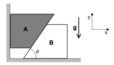
Use the following parameters in your analysis:  $m_A = 160$  kg,  $m_B = 80$  kg and  $\theta = 30^{\circ}$ .
