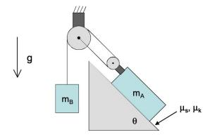
Use the following parameters in your analysis:  $m_A=40$  kg,  $m_B=80$  kg,  $\mu_s=0.3$ ,  $\mu_k=0.15$  and  $\theta=60^\circ$ .
