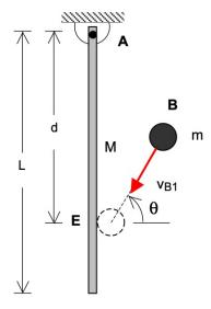
Use the following parameters in your analysis: L=3 m, d=2 m, m=10 kg, M=15 kg, e=0.6,  $\theta=60^{\circ}$  and  $v_{B1}=20$  m/s.
