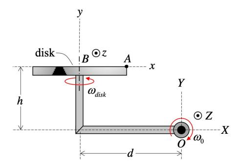
Use the following parameters in your analysis:  $\omega_0 = 4 \text{ rad/s}$ ,  $\omega_{disk} = 3 \text{ rad/s}$ , d = 18 cm, h = 10 cm and R = 6 cm.
