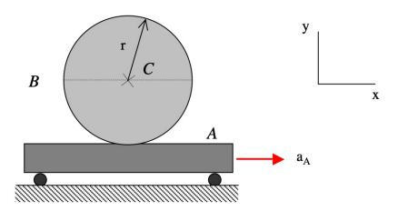
Use the following parameters in your analysis: r=0.6 m,  $v_A=8$  m/s,  $v_C=5$  m/s,  $a_A=-4$  m/s<sup>2</sup> and  $a_C=8$  m/s<sup>2</sup>.
