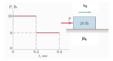
Use the following parameters in your analysis:  $v_0=2$  ft/s,  $\mu_k=0.3$  and t=0.4 s.
