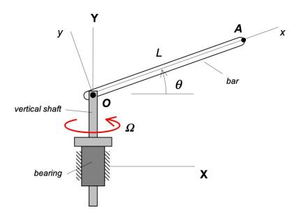
Use the following parameters in your analysis:  $\Omega=5$  rad/s,  $\dot{\theta}=4$  rad/s,  $\ddot{\theta}=-3$  rad/s<sup>2</sup> and L=2 m.
