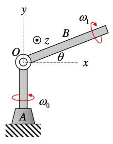
Use the following parameters in your analysis:  $\omega_0=4$  rad/s,  $\omega_1=3$  rad/s,  $\theta=30^\circ$  and  $\dot{\theta}=2$  rad/s.
