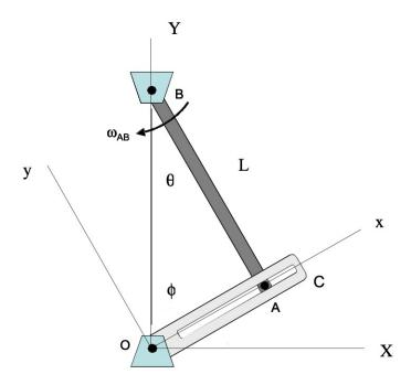
Use the following parameters in your analysis:  $\omega_{AB}=2$  rad/s, L=0.17 m,  $\theta=30^{\circ}$  and  $\phi=60^{\circ}$ .
