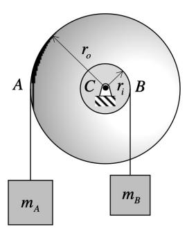
Use the following parameters in your analysis: M=10 kg,  $m_A=12$  kg,  $m_B=9$  kg,  $r_i=0.06$  m and  $r_o=0.2$  m.
