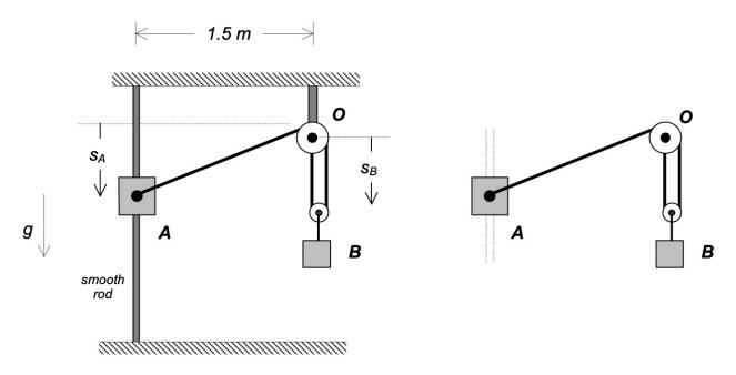
Use the following parameters in your analysis:  $m_A = 10$  kg,  $m_B = 10$  kg,  $v_{A1} = 5$  m/s and  $s_A = 2$  m.
