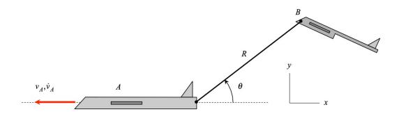
Use the following parameters in your analysis: R=80 m,  $v_A=600$  m/s,  $\dot{v}_A=5$  m/s<sup>2</sup> and  $\theta=30^\circ$  and  $\dot{\theta}=0.1$  rad/s.
