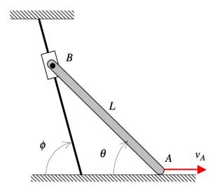
Use the following parameters in your analysis: L=2 ft,  $v_A=4$  ft/s,  $\theta=30^\circ$  and  $\phi=53.13^\circ$ .
