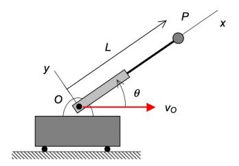
Use the following parameters in your analysis:  $\theta=90^{\circ}, v_O=6$  m/s,  $\dot{\theta}=5$  rad/s, L=2 m,  $\dot{L}=0$  m/s, and  $\ddot{L}=3$  m/s<sup>2</sup>.
