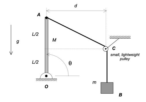
Use the following parameters in your analysis: m = 20 kg, M = 100 kg, L = 3 m and d = 4 m.
