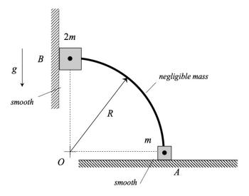
HINT: Note that AB is a two-force member. What does this say about the direction of the reaction forces on blocks A and B due to member AB?
