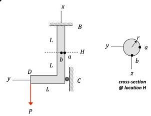
The L-shaped structural member above has a circular cross-section with a radius of r. The member is supported by a fixed connection to ground at B and a roller at C as it carries a downward vertical load of P at D. What is the absolute maximum shear stress in the member at points "a" and "b" on the cross-section at H? Expect the following steps in the analysis.
