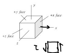
The three components of normal stress and the six components of shear stress shown on the body on the previous pages all correspond to positive quantities. These components on the positive faces, along with those on the negative faces, are shown on the stress cube below, where a "primed" quantities (e.g.,  $\sigma'_{x}$  and  $\tau'_{xy}$ ) are those components on the negative faces.
