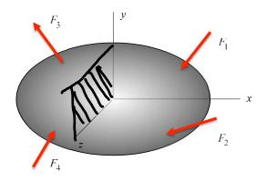
Making cut through body parallel to yz-plane:
