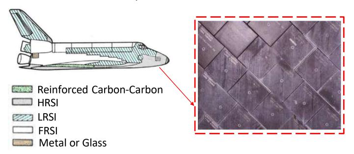
During re-entry, the space shuttle locally experiences temperatures up to , 1500 °C. The heat-protection tiles on the surface of the shuttle are designed to have a small thermal expansion coefficient, but gaps are still left between tiles to allow thermal expansion.
