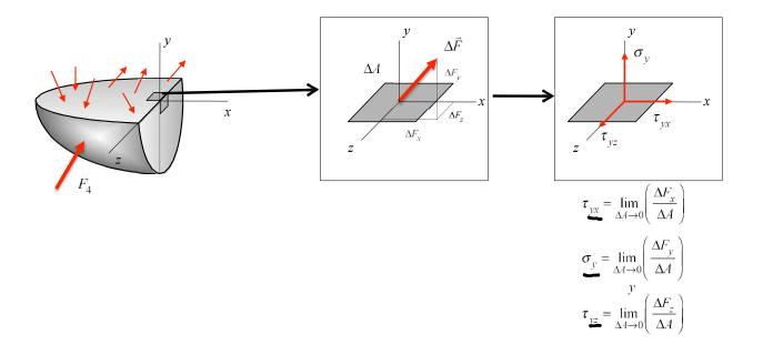
Making cut through body parallel to xy-plane:
