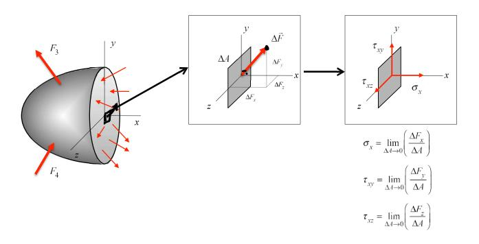
Making cut through body parallel to xz-plane:
