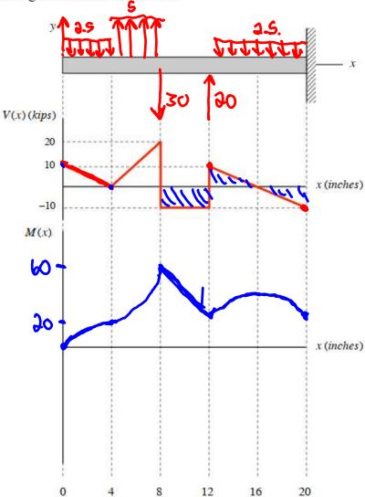
Draw the shear force and bending moment diagrams in the plot axes below for the loaded beam shown.
