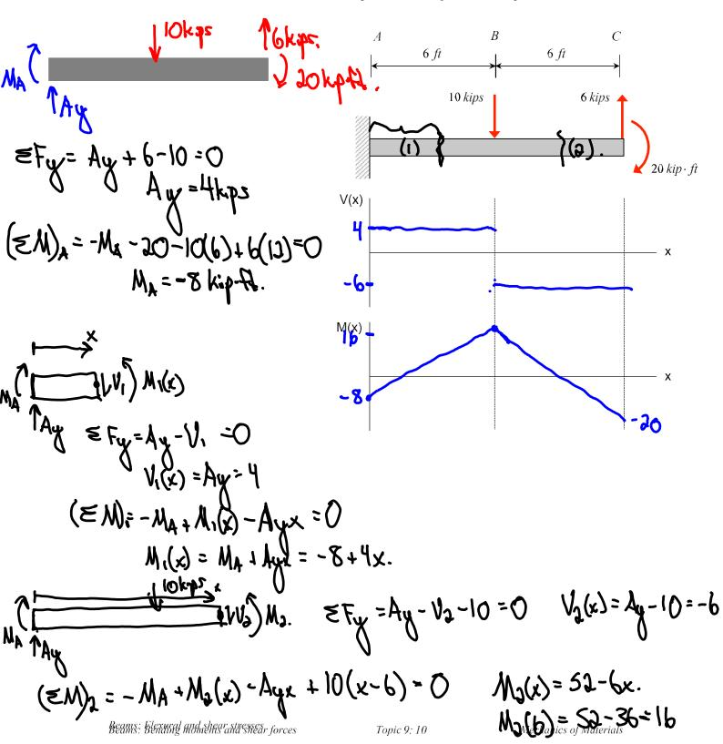
Two transverse forces and a couple are applied as external loads to the cantilevered beam AC. Draw the shear force and bending moment diagrams in the plot axes below.
