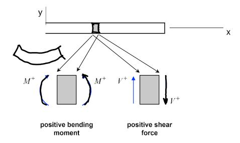
When making a cut through a cross section of the beam, the positive sign conventions for the bending moment and shear force are as shown below:
