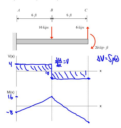
Consider the cantilevered beam shown below that is loaded only by concentrated and distributed forces (no external couples applied). The loading is not shown in the figure of the beam. The internal shear force distribution in the beam is shown below. For this beam:
