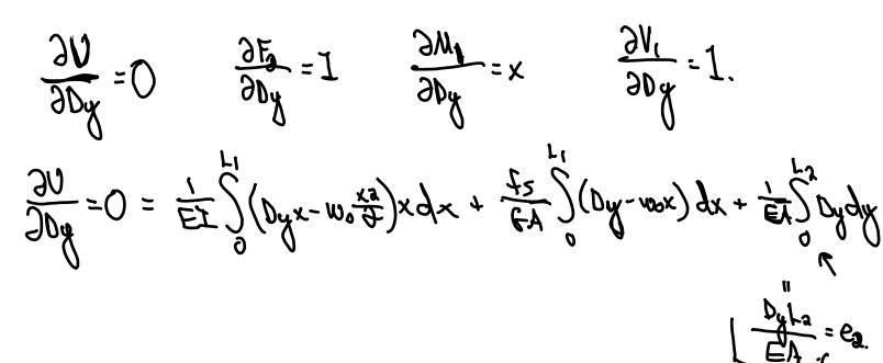
$$-\Theta = \frac{1}{EI} \int_{0}^{L_{1}} (Dyx - w_{0}\frac{x^{2}}{2}) \times dx + \frac{4}{GA} \int_{0}^{L_{1}} (Dy - w_{0}x) dx.$$
