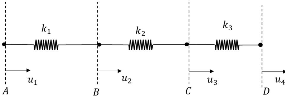
$$k_1 = \frac{E(A_1)}{L_1} = \frac{\pi d^2 E}{4L}; \quad k_2 = \frac{E(A_2)}{L_2} = \frac{\pi d^2 E}{2L}; \quad k_3 = \frac{E(A_3)}{L_3} = \frac{\pi d^2 E}{4L};$$
