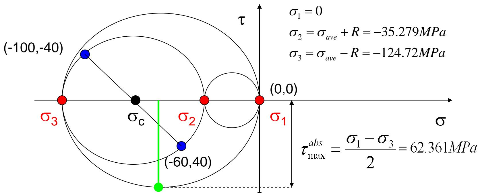
*Example 4: For the given stress state (a) Sketch Mohr's circle for three dimensional stresses (b) determine the absolute maximum shear stress.*
