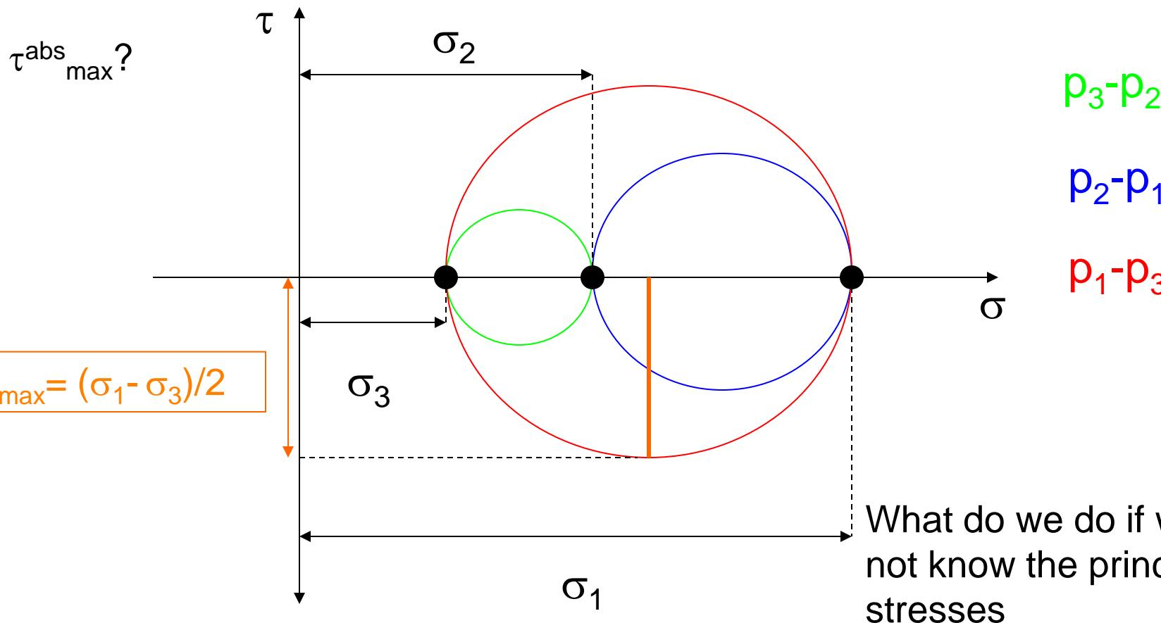
*Example 3: For the given stress state (a) Sketch Mohr's circle for three dimensional stresses (b) determine the absolute maximum shear stress.*
