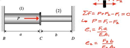
A structure is made up of axial members (1) and (2) shown above with a load of P acting at the rigid connector C. You are asked to re-design the structure by changing the length b of member (2) in order to decrease the normal stress in that member. You are <u>not</u> able to change any other aspect of the design such as the material or the cross sectional area of the member. Circle the answer below that describes best your design options.
