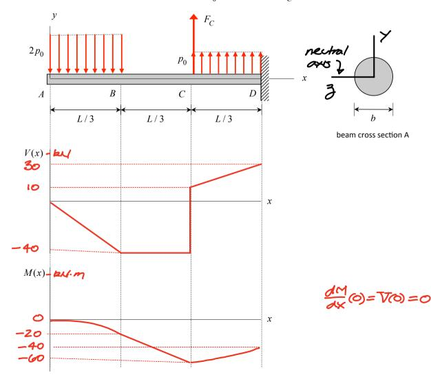
Use the following in your calculations: L = 3 m,  $p_0 = 20 kN / m$ ,  $F_C = 50 kN$  and b = 0.1 m.
