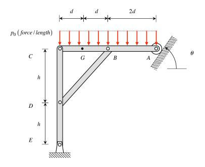
Determine expressions for the internal resultants F(x), V(x), M(x) at an arbitrary point X along AB.
