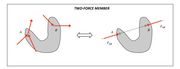
When drawing FBDs of structural components, it is convenient to take advantage of the simplicity of a two-force member when they exist. Trusses are made up exclusively of two-force members. Other structures, such as frames, contain two-force members along with members having more complicated boundary conditions.
