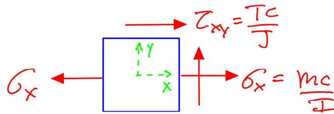
(ii) D.E. should have a smaller value for  $d$  since M.S.S. is more conservative failure theory.
