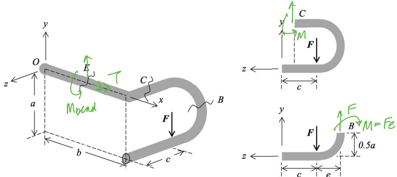
(i) For a cut through the handlebars at location *B*, the internal loads are
