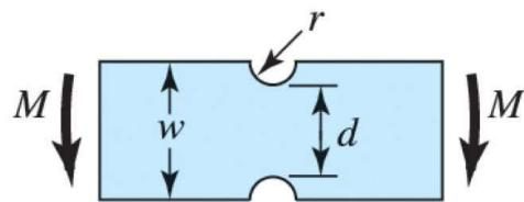
Determine the following for the notched rectangular bar loaded in bending.
