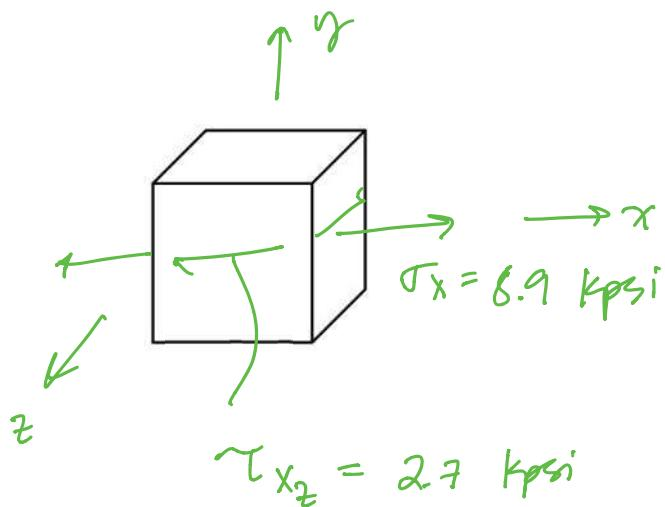
iv) the critical cross-section is at the wall because that is the location with the highest bending moment.
