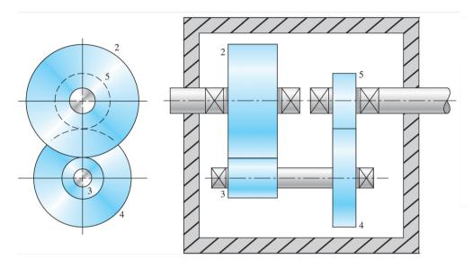
If gear 2 has 144 teeth and gear 3 has 18 teeth, find the numbers of teeth of gears 4 and 5.
