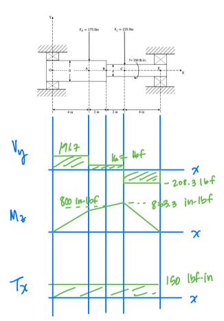
b) outical cross-section is at B due to relatively high bending moment and stress raiser.
