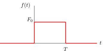
Consider a damped, single-DOF system with an equation of motion of:  $m\ddot{x} + c\dot{x} + kx = F(t)$
