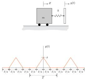
The undamped, single-DOF system above is given a base excitation of y(t). The base motion y(t) is *T*-periodic in time, as shown above.
