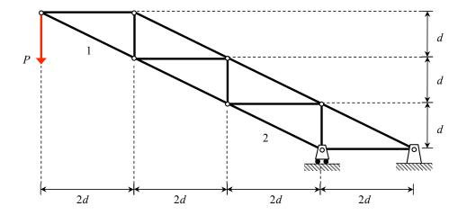
Determine the zero force members in the truss below. If you identify one zero force member ar a pin/joint use that in determining if there are other zero force members at the pin. Give the reasons why the identified member has no force.
