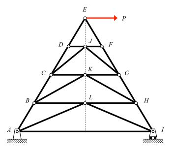
Given: A vertical load P is applied to the truss, as shown below.
