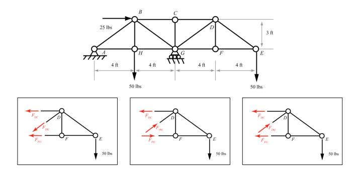
Given: A truss shown below is loaded with forces P, Q and R at joints B, H and E, respectively.
