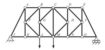
For the given loading, determine the zero-force members the truss shown. Give the reason.
