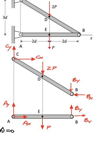
(1)  $\Sigma F_{x} = (x - B_{x}) = 0$ (2)  $\Sigma F_{y} = (y - B_{y})^{2} - 2P = 0$ (3)  $\Sigma M_{c} = -2P(2d) - B_{y}(4d) - B_{x}(3d) = 0$
