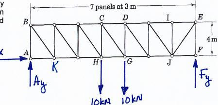
**b)** Calculate the reaction forces at supports A and F ( $\vec{F}_A$  and  $\vec{F}_F$ ) in vector form. (7 pts)
