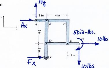
**b)** Determine the reactions at supports  $\bar{F}_A$  and  $\bar{F}_F$ . Express these reactions in vector form. (5 pts)
