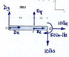
d) Determine the forces on member DEG at joints D and E. Express these forces in vector form. Remember to reference the free-body diagrams used in your calculations. (8 pts)
