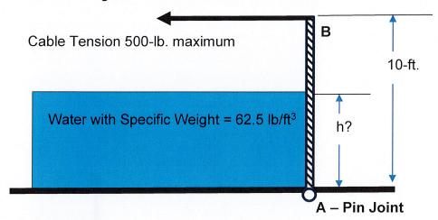
Hydrostatic Force = (Average Pressure/2)\*Area = (1/2)\* $\gamma$ \*h\*(h\*1) = 31.25\*h<sup>2</sup>
