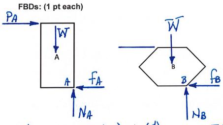
$\underline{ZM_{A}=0} = -P_{A}(2d) + W(\frac{d}{2})$   $\underline{ZM_{B}=0} = -P_{B}(1.4d) + W(d/_{2})$   $\therefore P_{A} = W/_{4} = 0.25 W$   $\therefore P_{B} = W/_{2.8} = 0.357 W$
