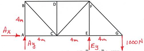
b) Calculate the reaction forces at supports A and E ( $\overline{F}_A$  and  $\overline{F}_E$ ). Write your answers in vector form. (6 points)
