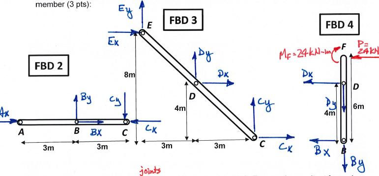
d) Solve for the internal forces at pins C and D on member EDC. Express the resultant forces in vector form.
