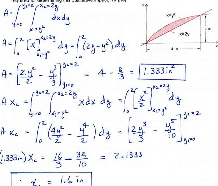
$$A = \frac{1.333 \text{ in}^2}{\text{2pts}} \qquad \text{(2pts)} \qquad x_C = \frac{1.6 \text{ in}}{\text{1 (2 pts)}}$$
