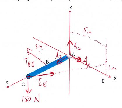
b) Write expressions for tension vectors T<sub>BD</sub> and T<sub>CE</sub> acting on the pole using their unknown magnitudes and known unit vectors. The applied load is shown as an example. Please express your result in reduced fractional form or decimal form. (4 pts)
