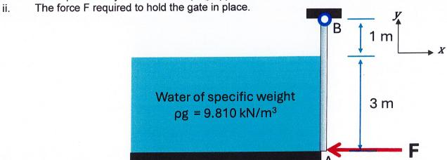
$$P_{A} = \rho gh = 9.81 \text{ kN} (3m) = 29.43 \frac{\text{kN}}{\text{m}^{2}}$$
