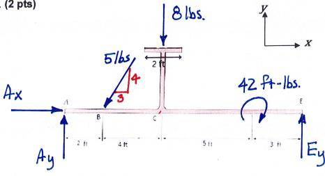
c) Clearly write the equilibrium equations and solve for the reactions at the pin support A and the roller support B. Express your solution in vector form. (12 pts)
