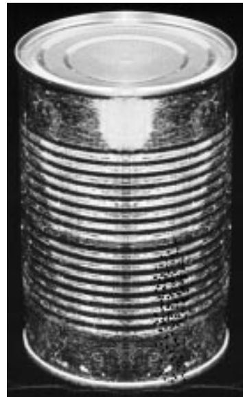
Pitted rust or leaking
