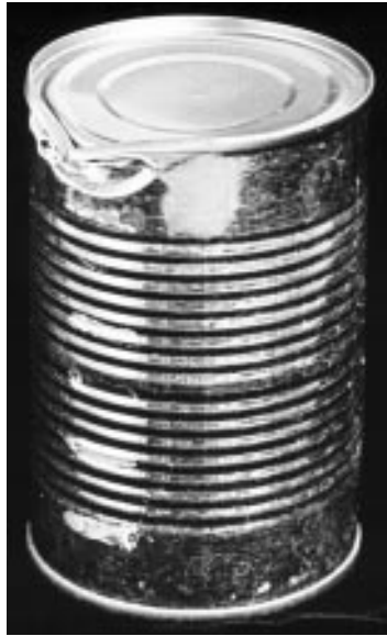
Dented at junction of side and end
