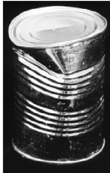
Sharp dent or dent on seam.
