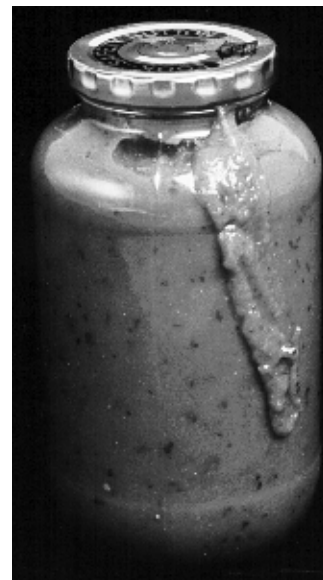
Leaking, crack or chips, or product discolored.
