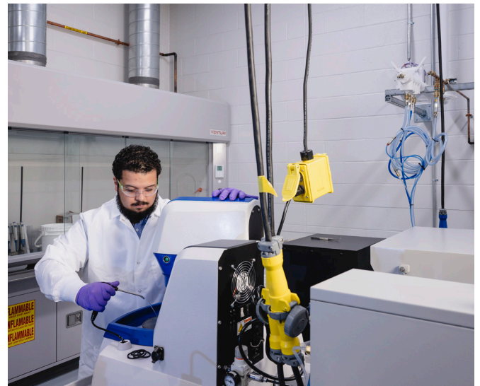
Julio Hernandez, a HAMTC engineer, implements a refined grinding and polishing regimen, crafting mirror-like finishes that reveal the intricate details under the lens of optical microscopy. (Purdue University photo/Charles Jischke)
