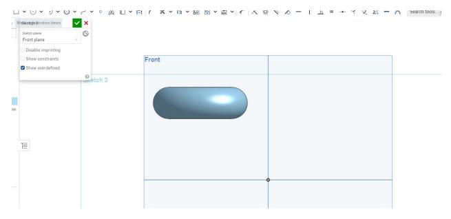
Draw a vertical line and then use arcs and lines to make another shape on the right side of the line. Be sure the shape attaches to the top and bottom of the vertical line. Your shape doesn't have to look just like mine but it does need to be a solid part sketch.
