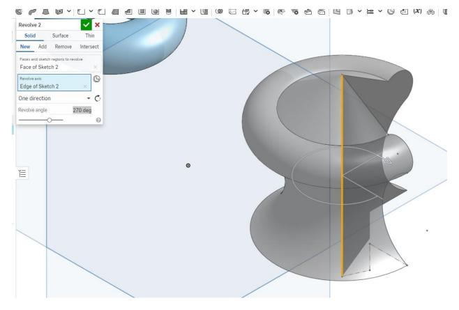
Use the Right mouse button to rotate the view and you will see the 270 degree Revolve.
