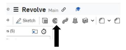
Left click on the circle and then left click on the Revolve axis to select the line to revolve around.
