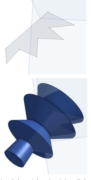
The Revolve axis does not always have to be vertical.
