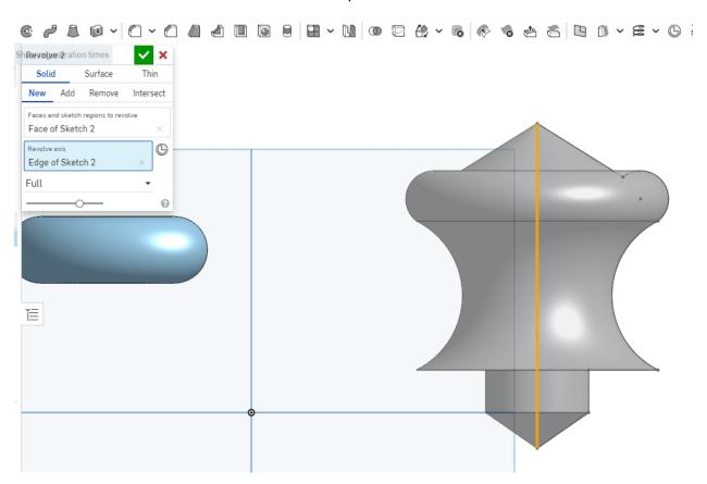
Select the Isometric view and reset the amount of Revolve to 270.
