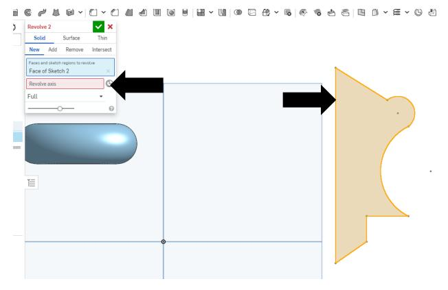
The sketch will Revolve around the axis with no space. This is a full Revolve but you can also set the amount of Revolve in the Full drop down menu.
