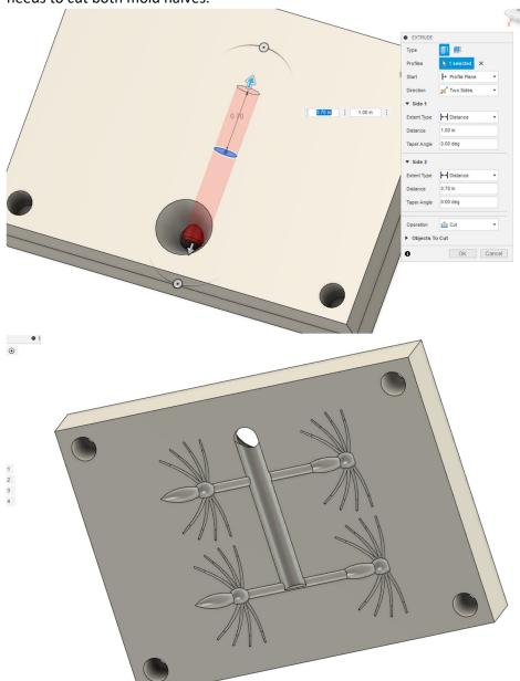
28. Air can get trapped inside the mold when plastic is injected into it. The last step is to create vents through the top to minimize bubbles. Create a sketch on the bottom of the top mold face. Vents at the end of each leg, tail, wing, abdomen, etc. are suggested. Vents should be a similar size or smaller than the feature to which they are attached. Using a pattern again might be helpful.
