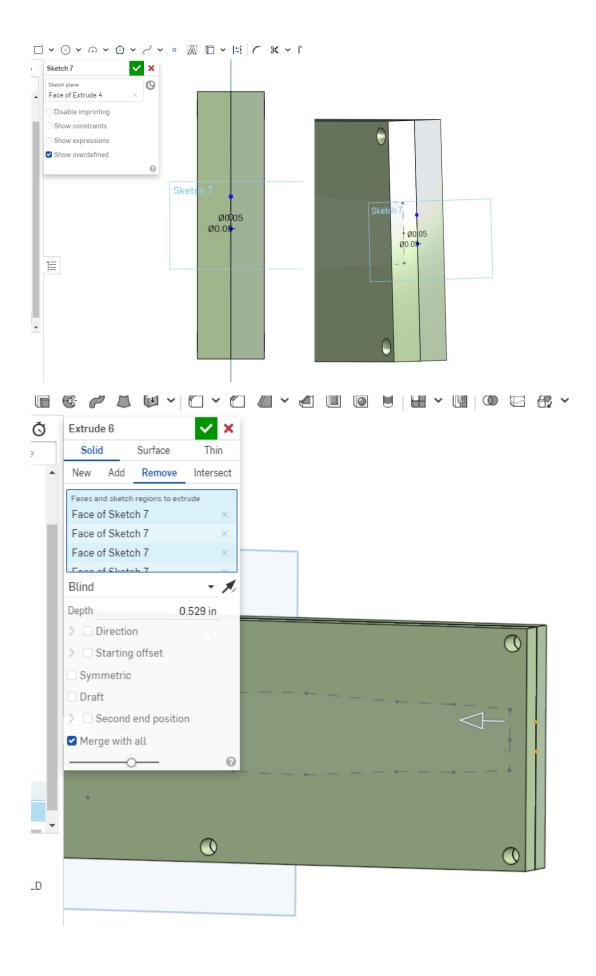
Hide one of the mold parts and rotate to see the small vent holes. Do the same with the other mold part to inspect the vent holes.
