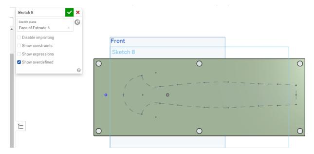
Select hole from the menu and use the counter sink with a diameter of .75". Follow the measurements on the menu. You can hide the bottom mold to confirm the counter sink hole.
