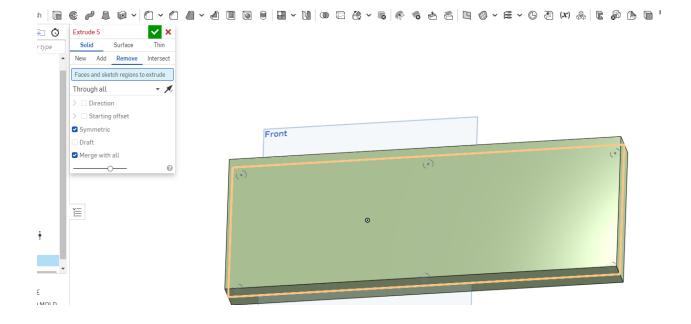
Rotate the part to confirm the holes go through both molds.
