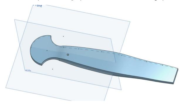
Start a new sketch with a rectangle on the plane you want to split the mold. This part will be split on the front plane.
