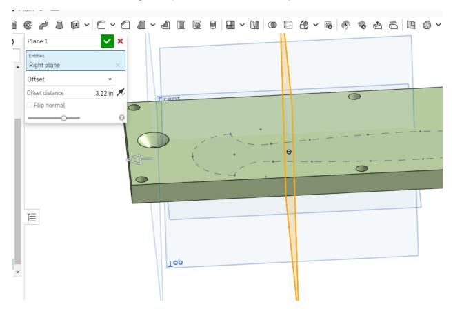
Draw a .25" circle on the plane. Finish the sketch and extrude the hole into the cavity. Follow the extrude menu to Remove and Merge with all so the extrude is in both parts of the mold.
