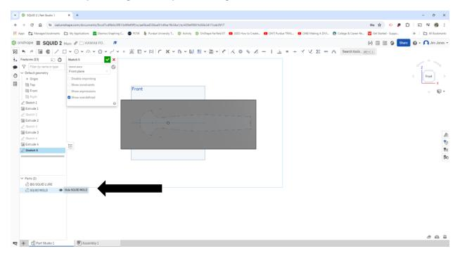
Start a new sketch on the same plane as the mold and draw a rectangle around the part. Click the green check mark to finish the sketch.
