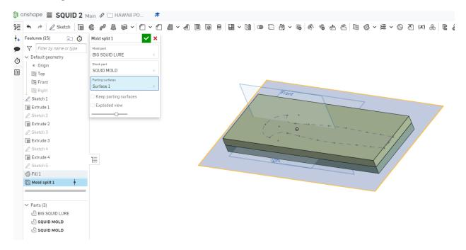
Select the Exploded view view box and set a distance and them click on the top surface of the mold to get an exploded view. The molds now have a cavity that will be where the plastic is injected. Click the green check mark and inspect your work.
