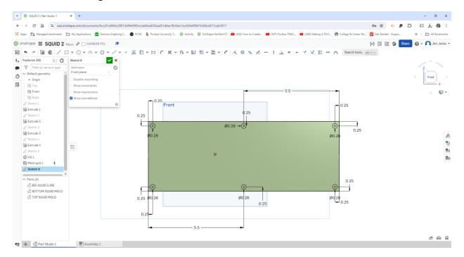
Extrude the holes Symmetrically to go through both molds and set Remove on the menu to create the holes through both molds. Click on Sketch 6 for the holes and the six holes will highlight. Select Merge with all from the Extrude menu and select through all in the drop down menu Click the green check mark.
