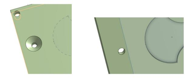
Add a construction plane to go through the hole to draw a .25" channel from the hole into the lure. This is needed to get the plastic into the lure cavity.
