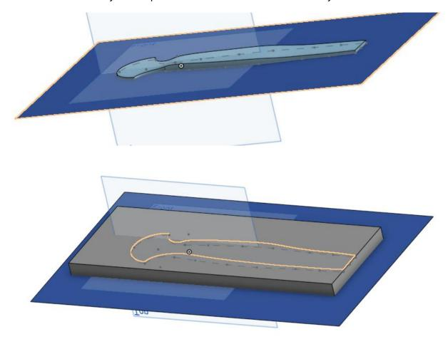
Select Mold Split on the menu bar. You may need to use the Search tools to find it. In the Mold Split menu box, pick the lure as the Mold part. It may help to hide the mold.
