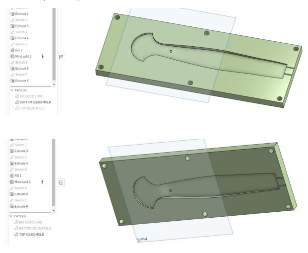
Start a new sketch on the top surface of the top mold. Draw a Point on the surface between the end of the mold and the lure. This point will be used to place a counter sink hole on the top mold as the opening for the plastic to be injected into the mold. Click the green check mark to finish the point sketch.
