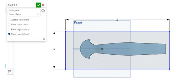
Complete the sketch the sketch and extrude symmetrically at 1 inch total. The extrude will need to be sized to the part so there is enough material around the part. Be sure to select NEW in the extrude menu to get a new part.
