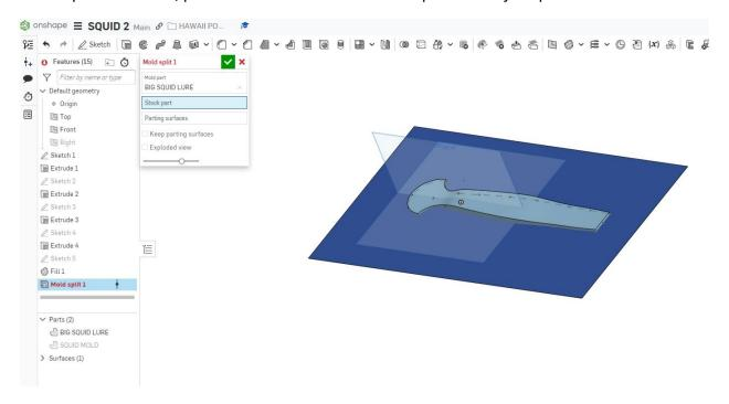
Unhide the mold and select the mold as the Stock part and then select the blue surface as the Parting surface.
