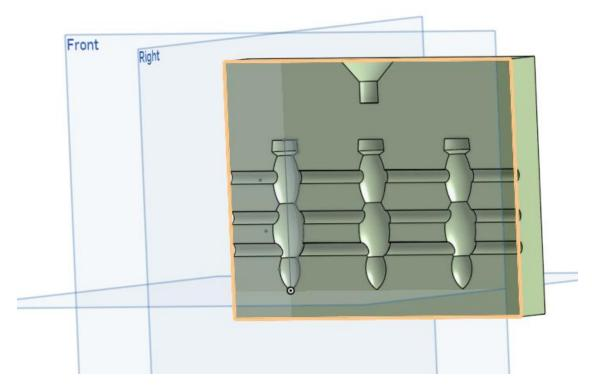
Start a new Sketch on the bottom of the molds to create the vent holes. Hide one of the molds and turn on the three lures to line up the circles.
