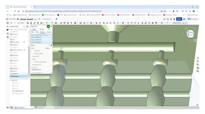
Unhide the other part of the mold and click the green check mark. Hide one part of the mold and check for the extrude. Hide all the planes.
