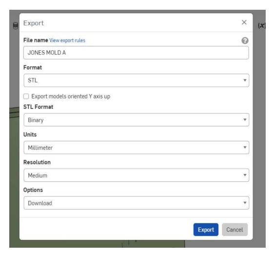
Do this for each part of the mold. The STL file will be used to slice the mold file into G code for the 3D printer.
