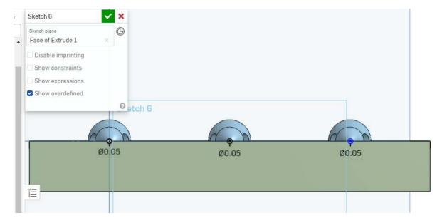
Turn on the molds and hide the lures. Finish the sketch. Extrude the holes into the lure cavity. When all parts of the circles are selected, finish the extrude.
