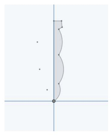
Select Revolve to create the lure a full 360 degrees. Use the vertical line as the axis. This should be New. Click the green check mark to complete the Revolve.
