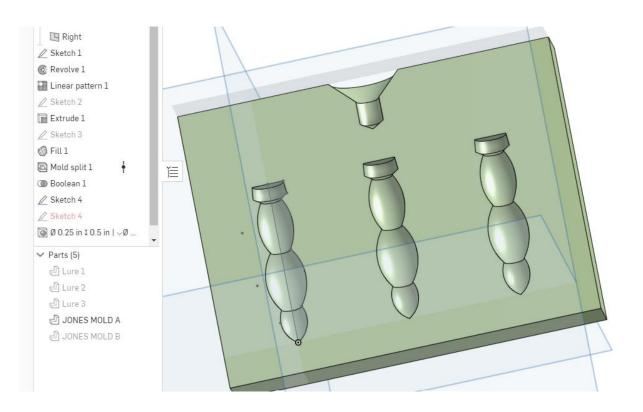
Start a new Sketch on the end of the molds to put in the channels for the skirt material for the legs. To draw the circles you can hide one side of the mold and unhide one of the lures to get the circles in the correct location. Unhide the mold and finish the sketch. I dimensioned the circles to 0.1".
