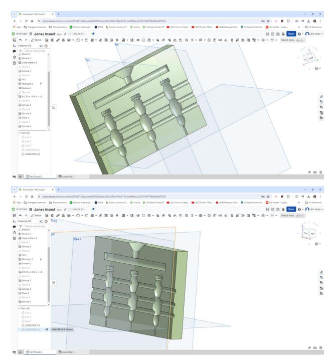
Create a new plane at the top of the three lures to create channels. Set the plane just below the top of the lures and click the green check mark.
