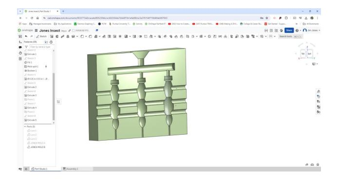
Start a new Sketch on the top of the mold surface. Draw four .28" circles to match the drawing. The center of each circle should be .25" from the two outside edges. These are the bolt holes. After sketching the circles click the green check mark. Extrude all four holes. Remove, Through All and Merge with all. Finish the extrude.
