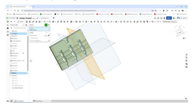
Make a new Sketch on the new plane and draw a .25" circle on the plane to create a channel above the three cavities. Unhide the other mold and one of the lures to line up the circle. Draw the circle and then tilt the mold to see if the circle is in the correct location.
