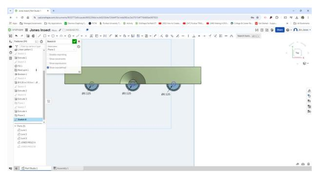
Extrude the three circles. Remove and set your distance so the extrude goes into the channel above. Select Merge with all.
