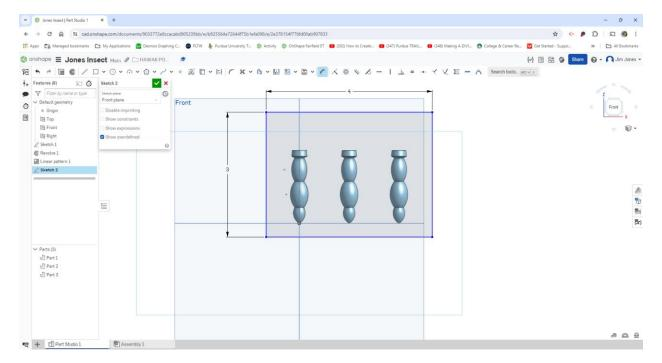
Extrude the rectangle making it a New extrude, Symmetric and 1" total thickness. Click the green check mark to complete the extrude.
