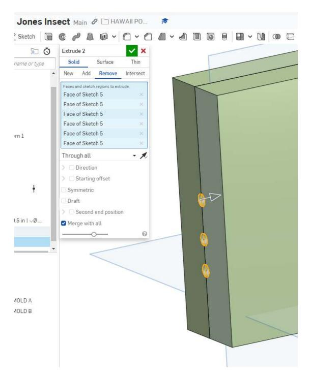
Finish the Extrude and check the molds.
