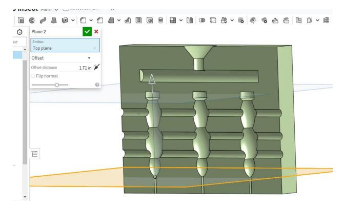
Start a new Sketch on the new plane. Unhide the three lures and draw circles at the center of each lure. Diameter should be .125". Finish the sketch.
