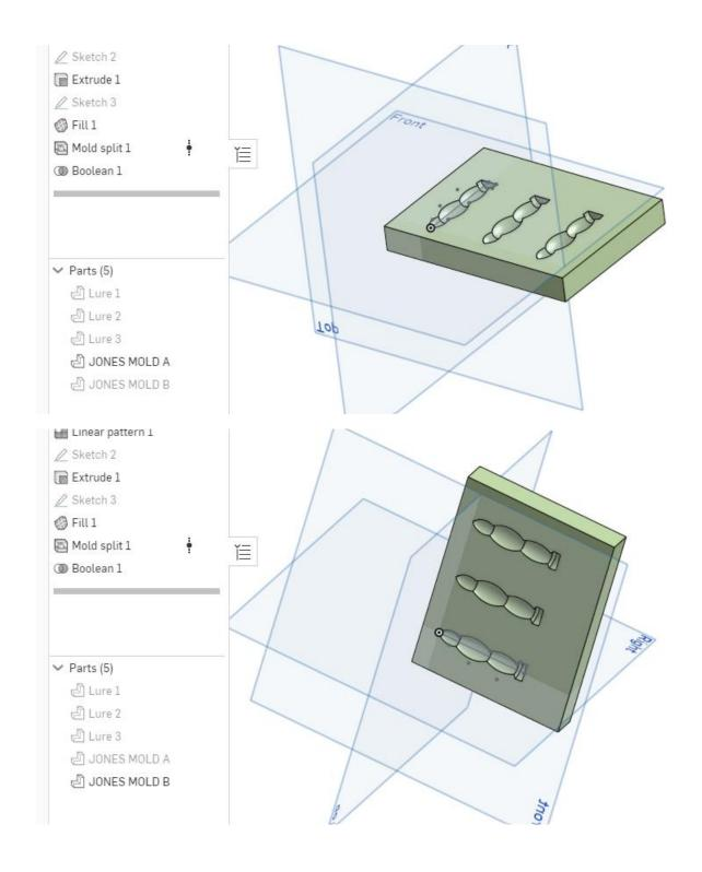
This mold will have channels for skirt material for legs and air vents. It will have a countersink opening on the top edge and it will need more channels on the inside for the hot plastic to fill the void.
