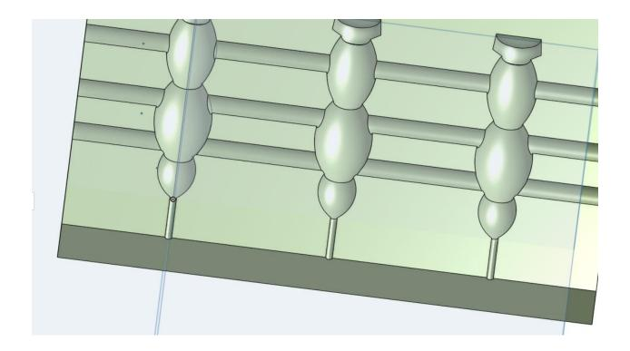
Now you need to add an offset plane through the center of the middle lure cavity and counter sink hole. Click on the plane icon and then select the Right plane and offset to the center. My Offset distance is 1.2" but yours may be different.
