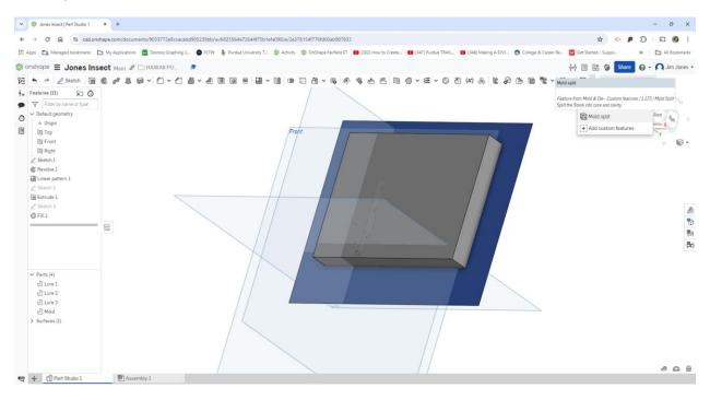
Click Mold part and click lure 1, Stock part click the Mold and Parting Surface click on the blue surface. Click on explode to see the separate parts. If explode does not work that is okay. You should have two mold parts and it is a good idea to Rename them at this time.
