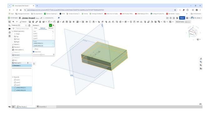
Hide the lures and the top half of the mold and you will see three lure cavities. Do the same for the other half of the mold.
