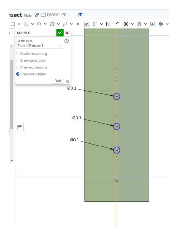
Extrude the three holes. Remove material and go all the way through. Click both parts of the circles to extrude in both halves of the mold. Besure to select Merge with all.
