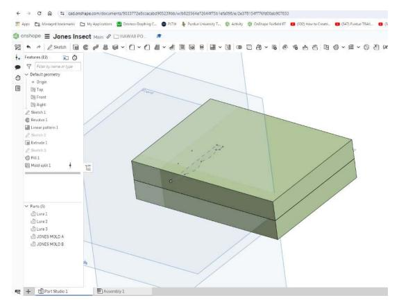
Hide the lures and the top of the mold and only one cavity shows in the mold. The next couple of steps will get the other two lure cavities to develop.
