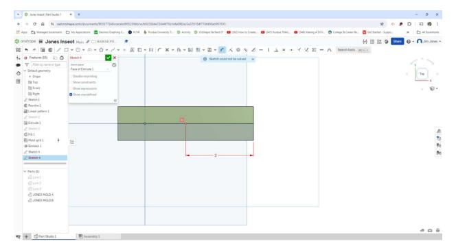
Select the Hole icon and use counter sink with the dimensions as shown. Finish the hole and check both parts of the mold for the counter sink.
