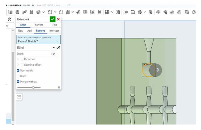
Extrude the circle and unhide the other part of the mold. Besure to select Remove, Symmetric and Merge with all. Distance should be 3". Click the green check mark and then confirm the channel goes over each lure. Hide and Unhide each part of the mold to confirm.
